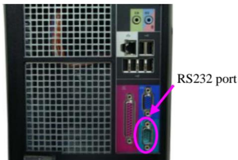
Connect the RS232 port of the ergometer to the RS232 port of the PC with an RS232 cable.
