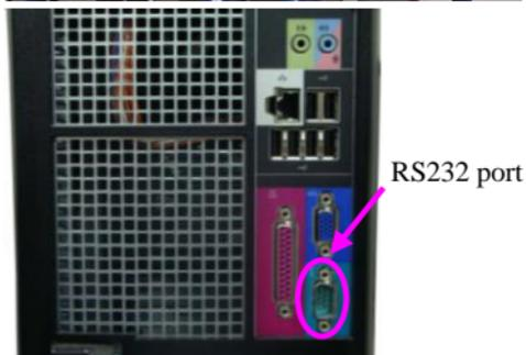
Connect the RS232 port of the treadmill to the RS232 port of the PC with an RS232 cable.
